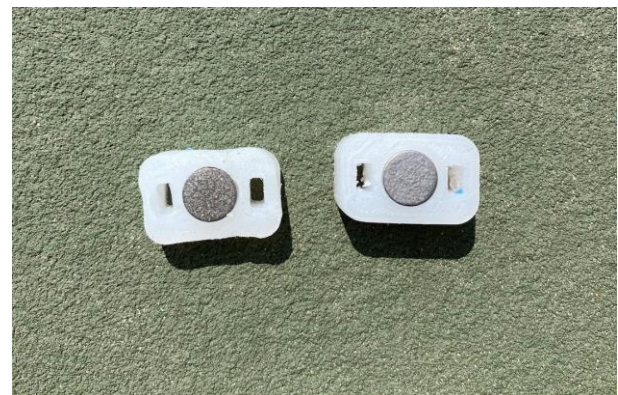
Figure 2. Final Damper Designs (3g left, 14g right)
