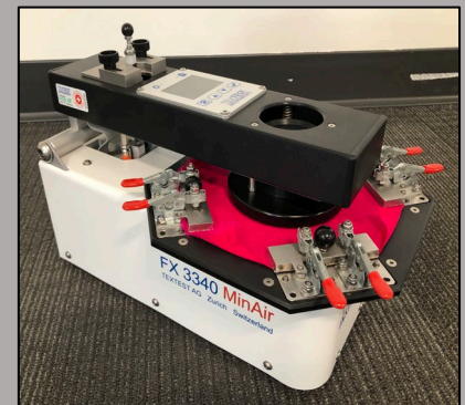
Fig. 1: Image of air permeability testing machine.
