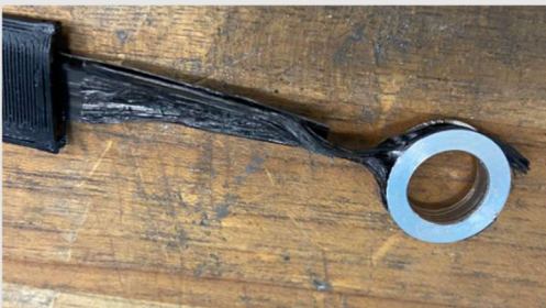
Figure 4: Tape Secured Around Bushing
