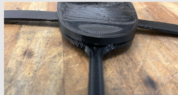
Figure 7: Integration of TPU Prints in the Insole Prototype
