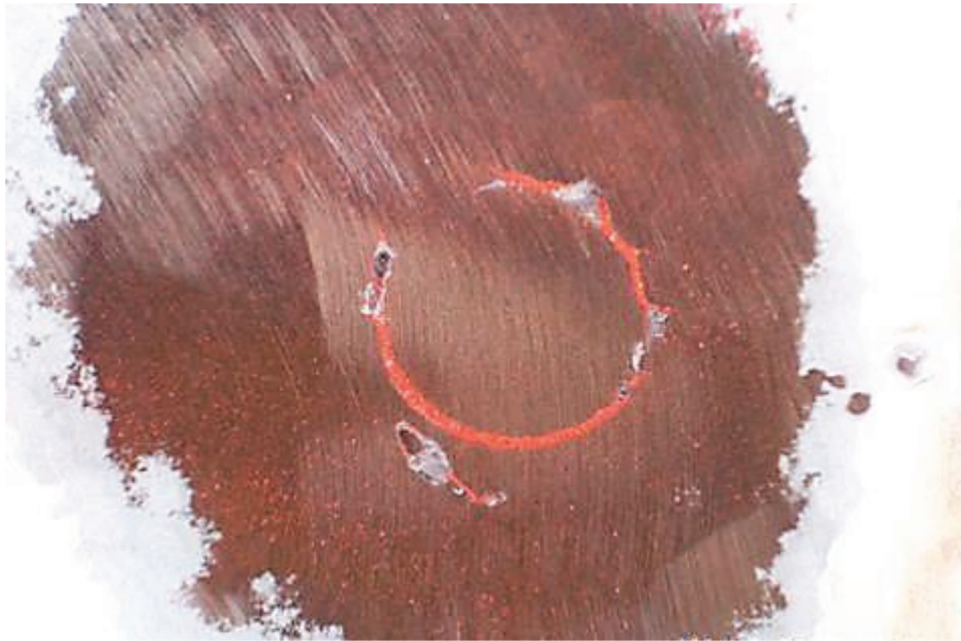
Figure 5.39 Magnetic particle test results at a plug weld showing lack of fusion defects (Photograph courtesy of Phil Fish).
