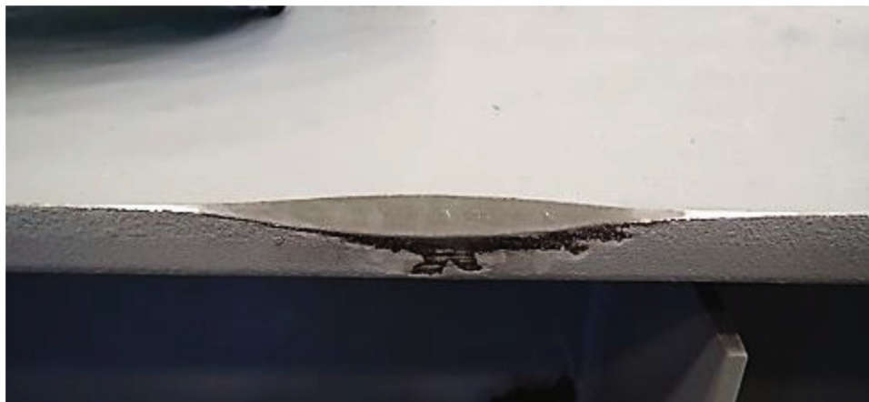
Figure 5.17 Example of edge flaw removed with 5:1 fairing ratio.
