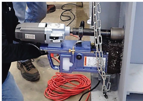
Figure 4.1 (Left) Example of magnetic-based drill, (Right) Annular cutter used for hole drilling.
