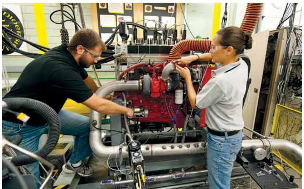
Purdue doctoral students Dan Van Alstine and Karla Stricker, who now works at the Cummins Technical Center, work on a diesel-engine test platform at the Ray W. Herrick Laboratories. The work is related to a new effort aimed at cutting fuel consumption in half for commercial vehicles by perfecting hybrid technologies for the world's burgeoning bus and truck fleets. The new Hoosier Heavy Hybrid Center of Excellence is funded with a $1 million grant from the U.S. Department of Energy's Graduate Automotive Technology Education initiative. (Purdue University photo/Mark Simons)
