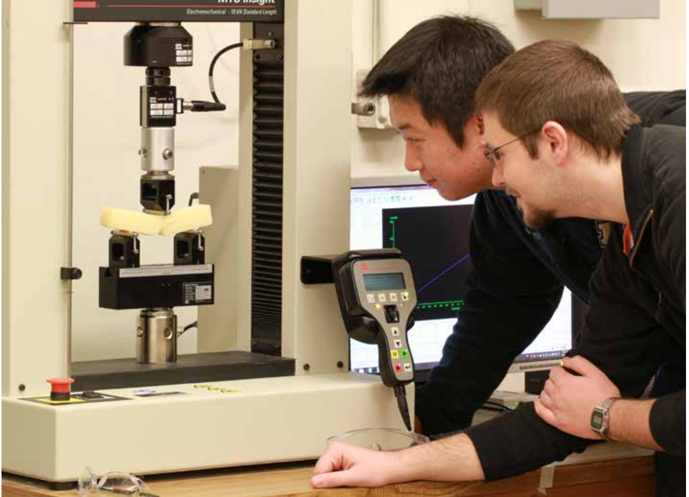
Nobphadon Suksangpanya (left) and Michael Jones supervising a fracture test being performed on a 3-D printed bioinspired helicoidal composite.
