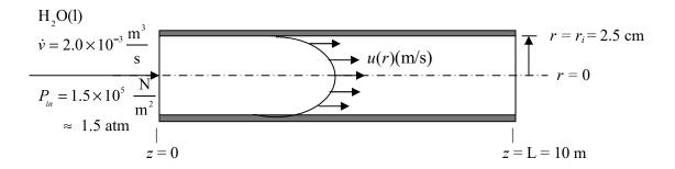
Water enters a 5.0-cm ID x 10.0 m long pipe at a volumetric flow rate  $\dot{v}=2.0 \text{x} 10^{-3} \, \text{m}^3/\text{s}$  and a pressure  $P=1.5 \text{x} 10^5 \, \text{N/m}^2$  (150 kPa  $\sim 1.5$  atm). Our goal is to find out as much as we can about relations among system variables at steady state.
