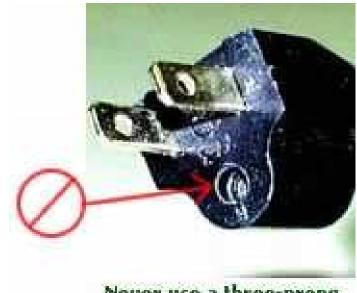
Never use a three-prong grounding plug with the third prong broken off.
