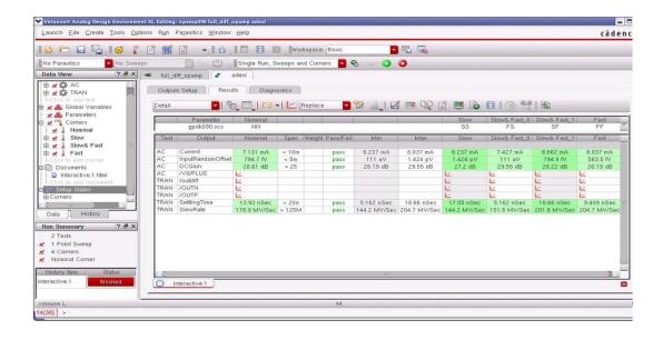
This screenshot shows the "default" view of ADE. The data view tree in the top-left is where the user describes their set up and simulations to be run, using other assistants not shown here. The table in the center shows the simulation results, with cell shading to report that the results have met the user's goals. This is a very small run: real runs will have hundreds of rows and thousands of columns and be distributed across hundreds of machines.
