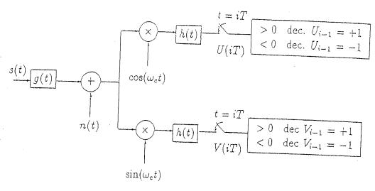
Each branch has a multiplier, a linear time-invariant filter, a sampler, and a threshold device. The baseband impulse response h(t) (with bandwidth much smaller than the carrier frequency  $\omega_c$ ) satisfies  $\infty$
