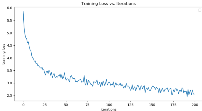
Figure: Loss vs. iterations during training over 100,000 random draws from a pool of 98,988 sentence pairs. This plot was produced by the script seq2seq_with_pretrained_embeddings.py in the Examples directory of DLStudio, version 2.0.9, with the learning rate set to 0.001.
