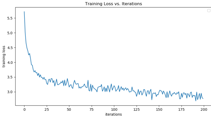
Figure: Loss vs. iterations during training over 100,000 random draws from a pool of 98,988 sentence pairs. This plot was produced by the script seq2seq_with_learnable_embeddings.py in the Examples directory of DLStudio, version 2.0.9, with the learning rate set to 0.001.
