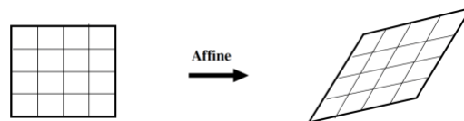
Fig. 3. Affine transform (straight and parallel lines hold their behavior after the transform)
