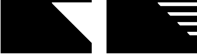
Fig. 5. Results of convolving the space-time plots with the transfer function defined in Section II. (Left) Full frame insertion and (right) black data insertion.
