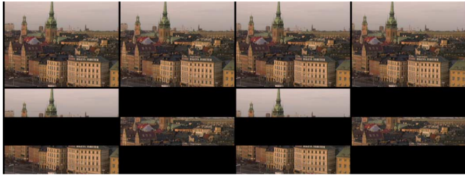
Fig. 7. A video sequence, with frame rate doubled by [top] full frame insertion, [bottom] black data insertion.
