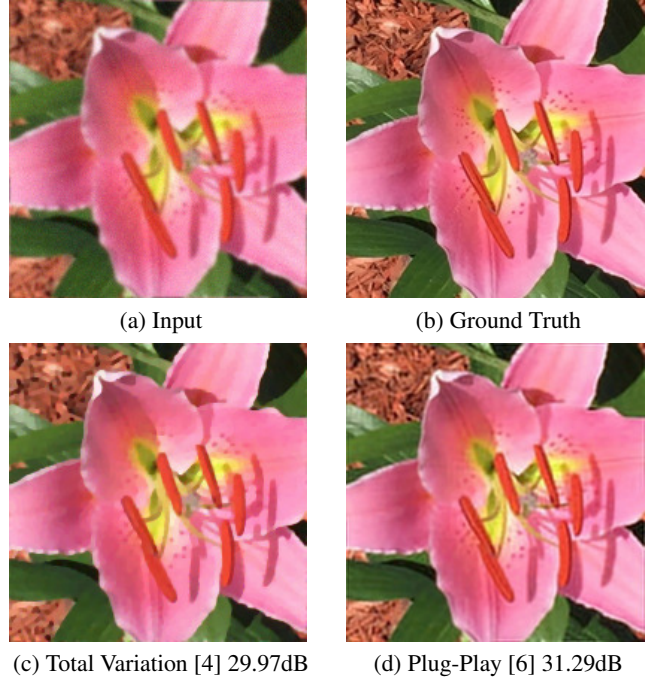
Fig. 1: Image deblurring using Plug-and-Play ADMM with BM3D denoiser compared to conventional ADMM with total variation (TV) prior. In this example, the regularization parameter is optimally tuned to \lambda = 10^{-4} for Plug-Play, and \lambda = 5 \times 10^{-3} for TV. The internal parameter of Plug-Play is \rho = 1 . The blur in this example is Gaussian of size 9 \times 9 with radius \sigma = 1 . The noise level is 5/255 .
