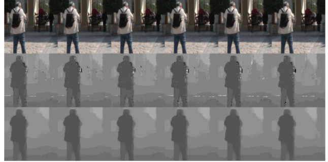
Fig. 1. Disparity Refinement for Old Timers. Top: Stereo Left View. Middle: Initial Disparity Estimate. Bottom: Processed Spatio-temporally Consistent Estimates.
