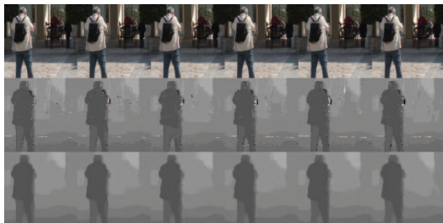
Fig. 2. Disparity map estimation result of “Old Timers” sequence. Top row: stereo video input (left view). Middle row: initial map estimation using loopy belief propagation [10]. Bottom row: result of applying deconvtv to the middle row. Parameters are \mu = 1 , (\beta_x, \beta_y, \beta_t) = (1, 1, 2.5) .
