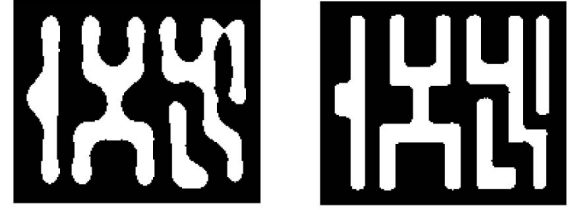
(a) Output binary image, using original pattern as mask (b) Output binary image, using proposed algorithm
