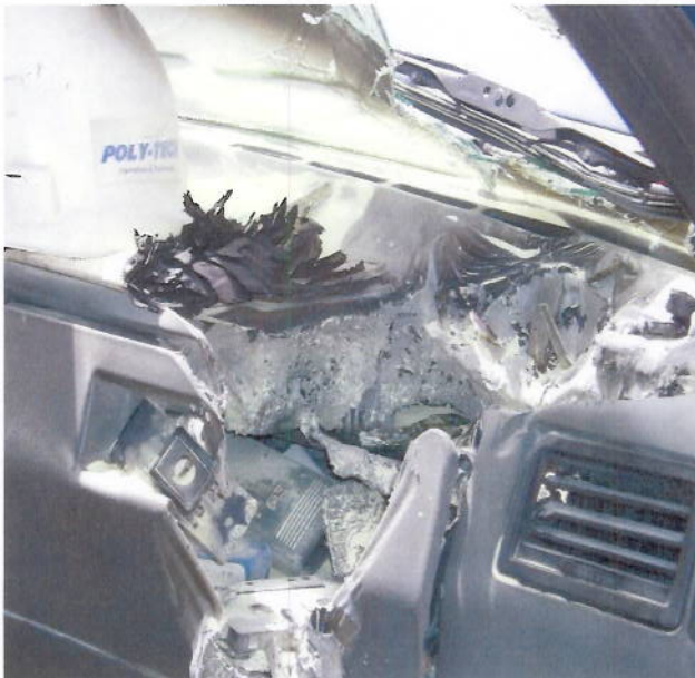
Figure 5: Evidence of rupture and heavy melting due to intense temperature as a consequence of the explosion
