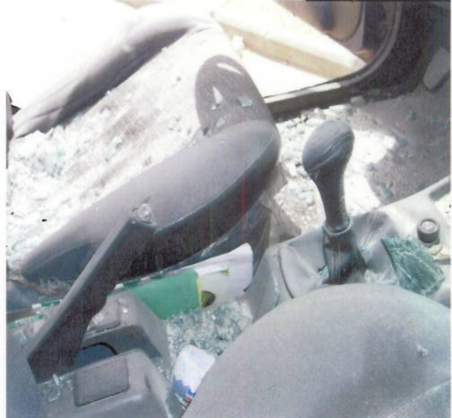
Figure 6: Car compartment damages and mobile phone units were destroyed beyond repair.
