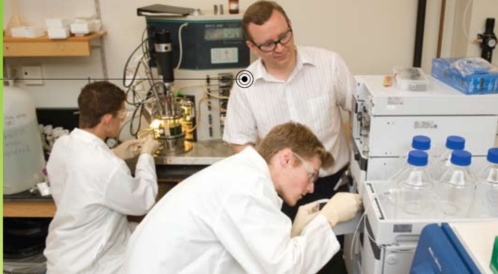
John Morgan (standing, center), and graduate assistant John O’Grady (left) set up the liquid chromatograph/mass spectrometer for analysis of the metabolism of algae cells. In the foreground, Cameron Hill, graduate research assistant, samples the photobioreactor.
