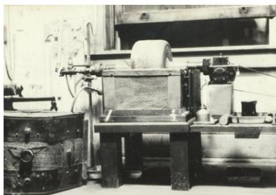
**Above:** One of the earliest pieces of equipment used in R.N. Shreve's work in 1932. A wrought iron ball mill used for the preparation of sodium amide by Abraham H. Goodman (M.S. '33).
