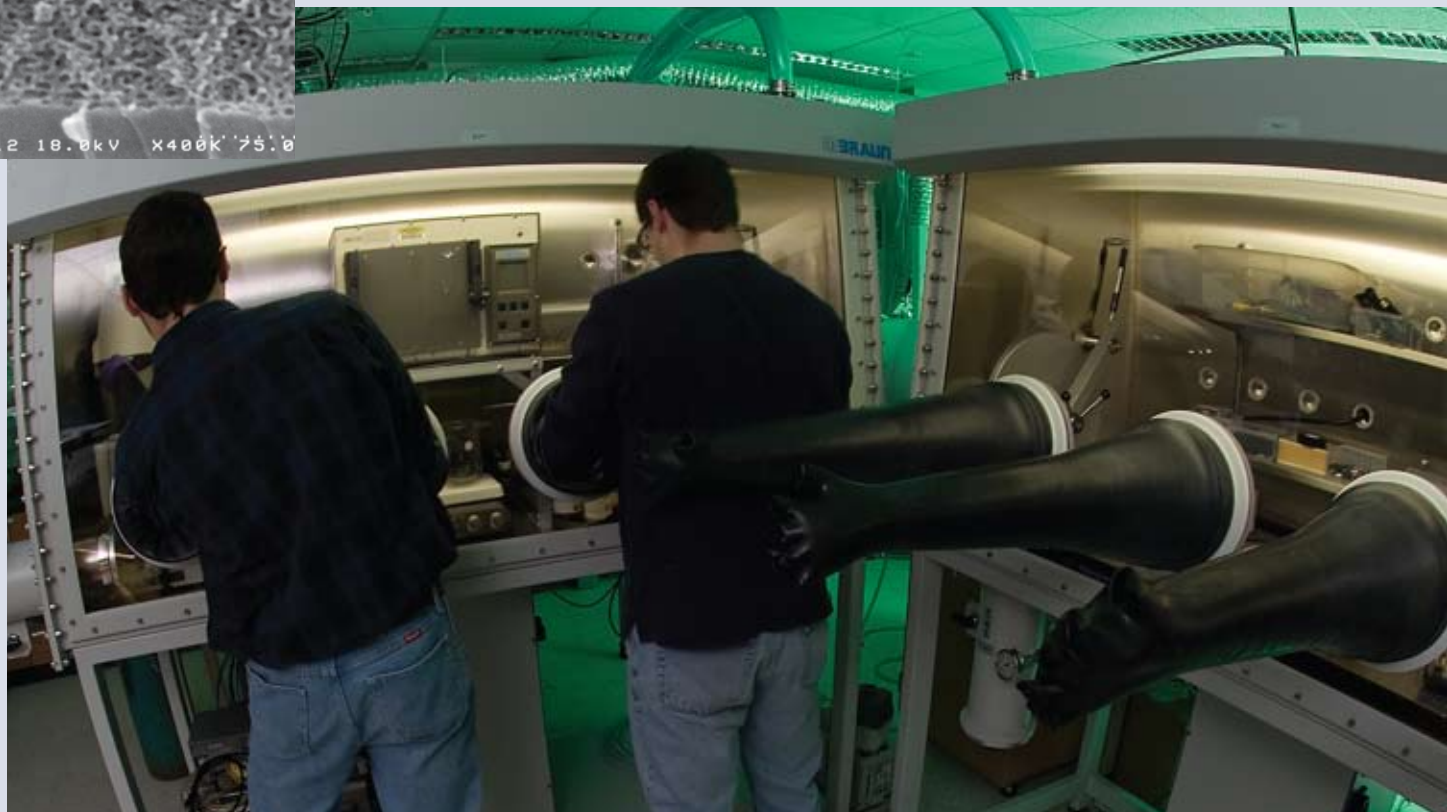
Standing outside this glove-box system’s oxygen-free, water-free, dust-free environment, students fabricate double-gyroid thin films for use in solar cells. Above: A double-gyroid film is represented in red. At 30 atoms wide, it is not visible to the naked eye. The gray image shows a greatly magnified cross section of a double-gyroid thin film.
