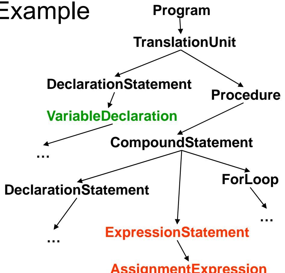
BreadthFirst traversal can be used to traverse upper-level objects in the IR before proceeding to lower-level objects
