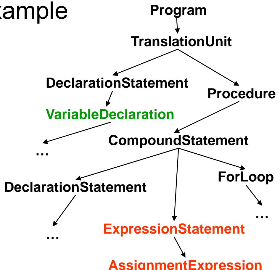
DepthFirst traversal can be used to find outermost loops in a procedure, including those inside compound statements.
