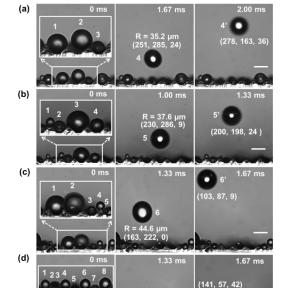
Selected cases showing droplet jumping induced by the coalescence of (a-d) three, four, five and eight droplets (marked with numbers in the inset images), respectively.
