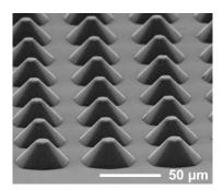
Hierarchical superhydrophobic surface
