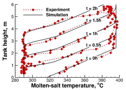
Model validation with experimental data recorded during a discharge (Pacheco, *JSEE*, 2002)
