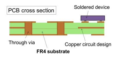
Requirements for substrate: electrically insulating, mechanically strong, low dielectric constant, high dielectric breakdown strength, good manufacturability
