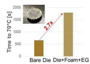
As an example, combining high conductivity foams and expanded graphite microflakes with a traditional paraffin wax phase change material significantly improves thermal performance during *in situ* tests.
