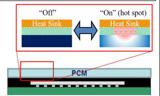
Schematic illustrating possible integration location of the PCM at the chip level to alleviate hot spots. During intense heating, the PCM changes phase absorbing energy at a nearly constant temperature.
