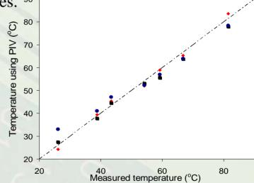
Plots shows the measured temperature vs the actual temperature. Uncertainty involved in the method is ±1 K.
