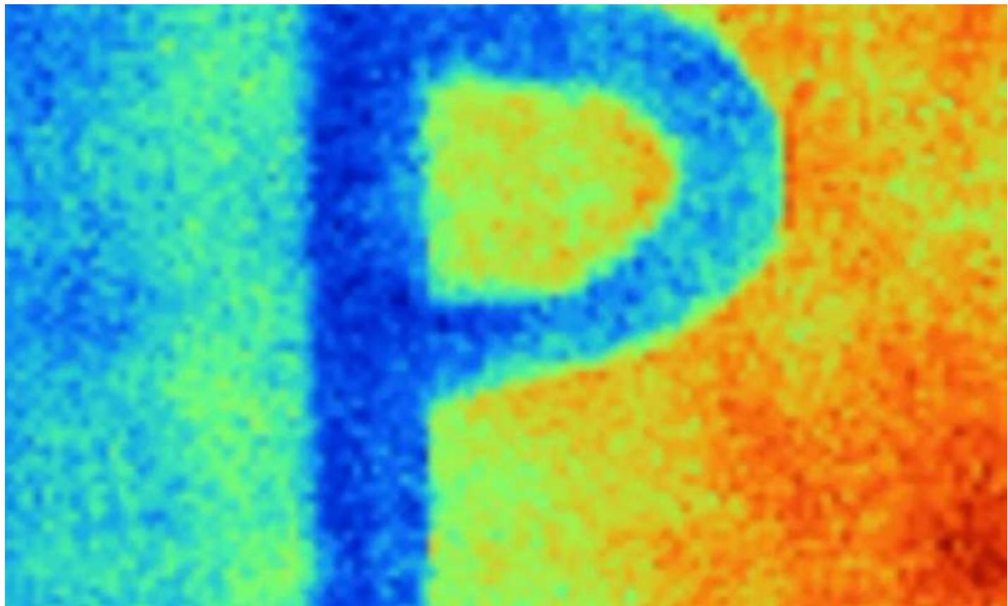
This infrared image shows that the P pattern painted with the Purdue radiative cooling paint is much cooler than the background painted with commercial paint. Credit: Xiangyu Li, PhD student of the School of Mechanical Engineering at Purdue University
