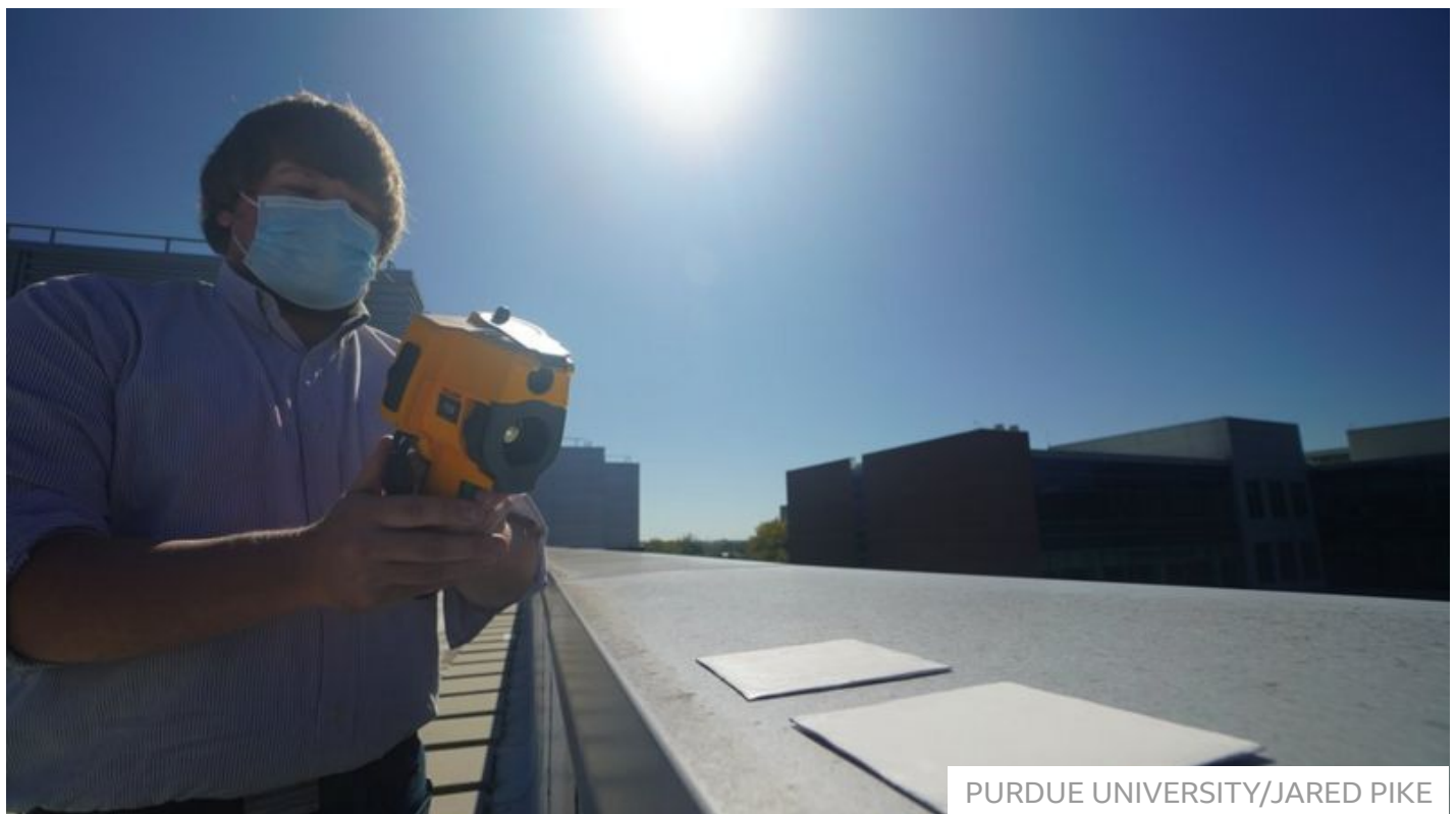
A Purdue researcher uses an infrared camera to compare the cooling performance of white paint samples
