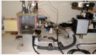
Nanowick supercooling system for 'power electronics'
