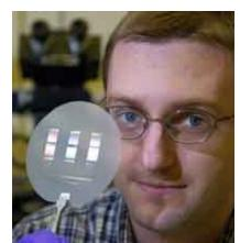
Engineers at Purdue University have developed a tiny "micro-pump" cooling device small enough to fit on a computer chip that circulates coolant through channels etched into the chip.
