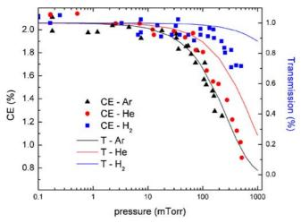
**FIGURE 7** The variation with CE with buffer pressure is given. The *symbols* represent the experimental data points and the *curves* give the 13.5 nm transmission (T) at different gas pressures for a path length of 78 cm
