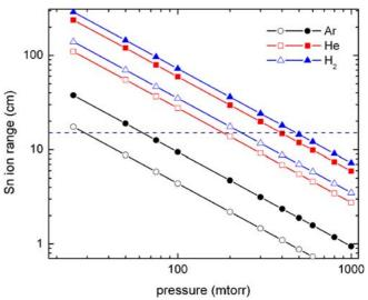
FIGURE 2 The SRIM estimate of the flight range of tin ions with different values of initial energies propagating into an ambient gas is shown. The hollow symbols correspond to a starting energy of 1 keV and the darkened symbols are for 5 KeV. The dashed line in the center corresponds to the Faraday cup position (15 cm)
