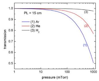
FIGURE 1 Transmission of 13.5 nm radiation at different argon and helium pressures is given for a path length of 15 cm
