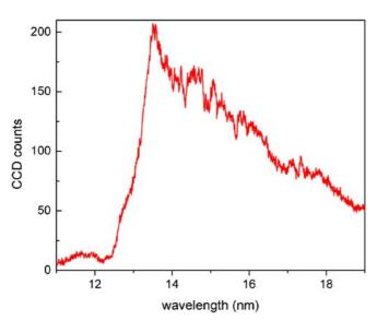
FIGURE 3  $\,$  UTA from laser produced Sn plasma. The laser intensity used is  $4\times10^{11}~W~cm^{-2}$
