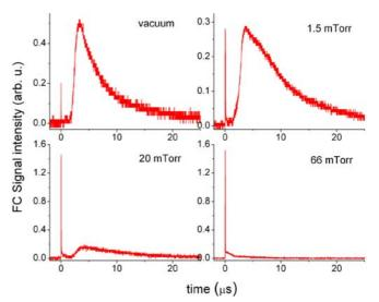
FIGURE 5 The TOF profiles of tin ions at different argon pressures are given
