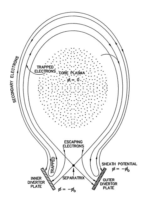
Fig.1 Schematic illustration of electron population in a collisionless SOL between inner and outer divertor plates in a tokamak device
