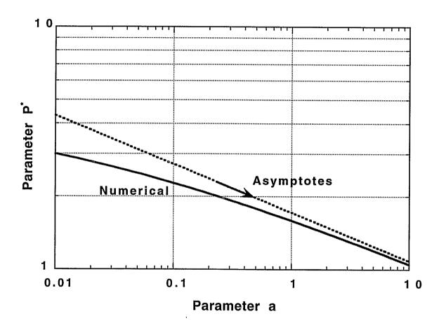
Fig. 7 Dependence of boundary momentum P on the tokamak parameter a.
