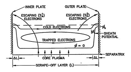
Fig.2 Schematic view of different electron populations in SOL described in the used model
