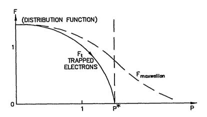
Fig.5 Distribution function of trapped electrons in SOL, compared to a Maxwellian distribution function
