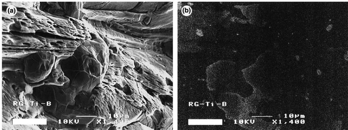
Fig. 6. (a) Surface modification, cracks and pore formations in RG–Ti–B recrystallized graphite during plasma irradiation ( $E_{\text{inc}} = 30 \text{ MJ/m}^2$ ,  $\tau_{\text{pulse}} = 360 \mu\text{s}$ ,  $T_{\text{preheat}} = 1200^\circ\text{C}$ ); (b) distribution of doped elements.
