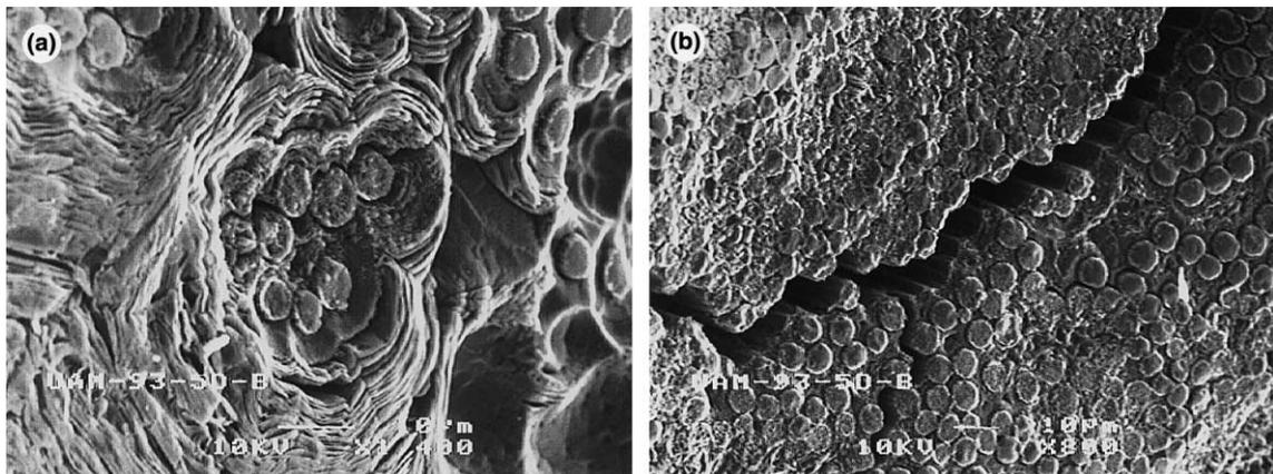
Fig. 3. (a) Surface modification and (b) crack formation of UAM-type carbon composites during plasma irradiation.
