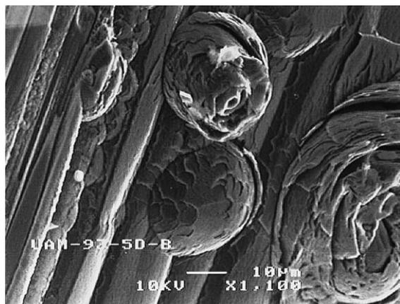
Fig. 4. Surface recrystallization and new structure formation for CFC materials during plasma irradiation.
