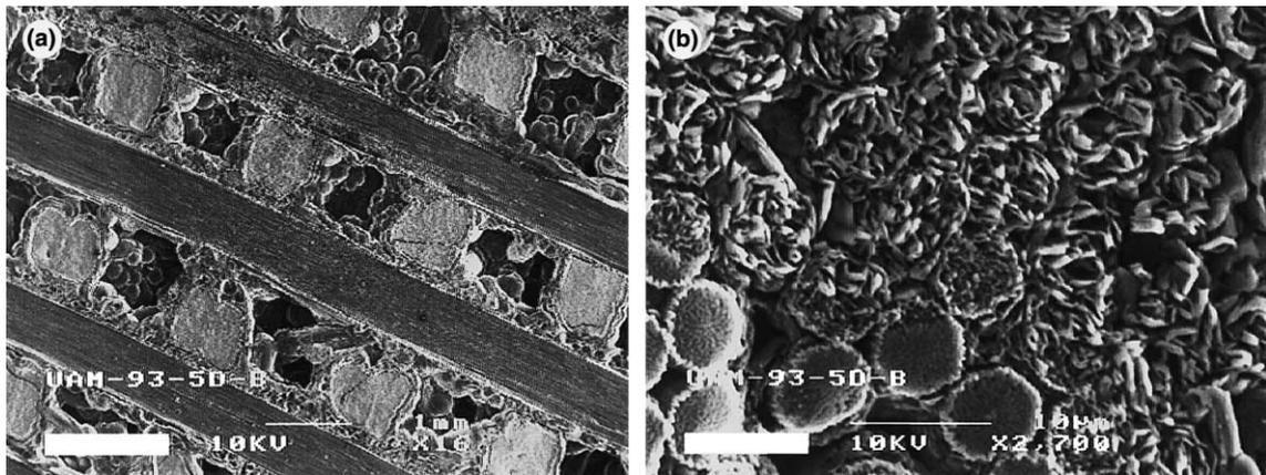
Fig. 2. Surface modification and pore formation in UAM-93-5D-B carbon composite during plasma irradiation at VIKA facility ( $E_{inc} = 30 \text{ MJ/m}^2$ ,  $\tau_{pulse} = 360 \text{ }\mu\text{s}$ ,  $T_{preheat} = 1200^\circ\text{C}$ ).
