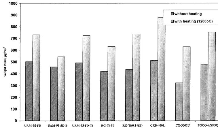
Fig. 1. Thermal erosion of various carbon-based materials after plasma irradiation at VIKA facility with and without preheating ( $E_{inc} = 30 \text{ MJ/m}^2$ ,  $\tau_{pulse} = 360 \text{ }\mu\text{s}$ ,  $T_{preheat} = 1200^\circ\text{C}$ ).
