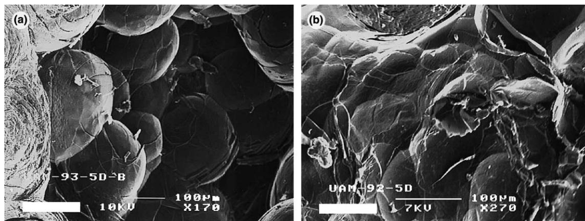
Fig. 5. (a) Spheroid formation on surface of CFC materials and (b) destruction during plasma irradiation ( $E_{\text{inc}} = 30\ \text{MJ/m}^2$ ,  $\tau_{\text{pulse}} = 360\ \mu\text{s}$ ,  $T_{\text{preheat}} = 1200^\circ\text{C}$ ).
