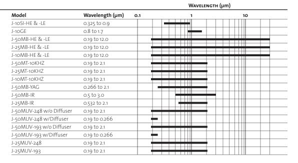
EnergyMax sensors are based upon pyroelectric technology and can therefore measure lasers at high repetition rates. The maximum repetition rate is primarily dependent upon the thermal resistance of the coating and the maximum pulse width the sensor is designed to measure. Refer to the summary table on page 6 for maximum laser pulse width limitations.
