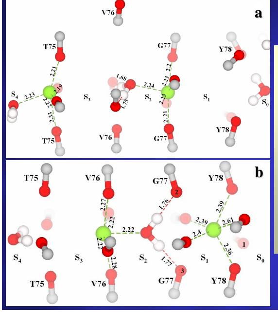
> Size selectivity: ionic size matters. K<sup>+</sup> ions fit comfortably in their binding sites without deforming the SF. The Na<sup>+</sup> binding cavity is smaller; the SF deforms providing five coordinating ligands to favorably cradle Na<sup>+</sup>. SF collapse around Na<sup>+</sup> locally occludes the conduction pathway.
