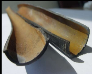
HDPE Pipe (Iron coated)
