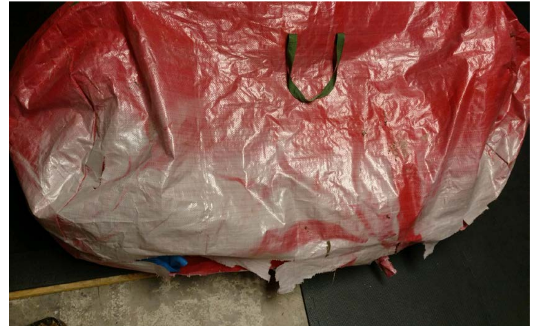
Photo of a Nylon bag under a deck for ½ summer showing light induced aging
