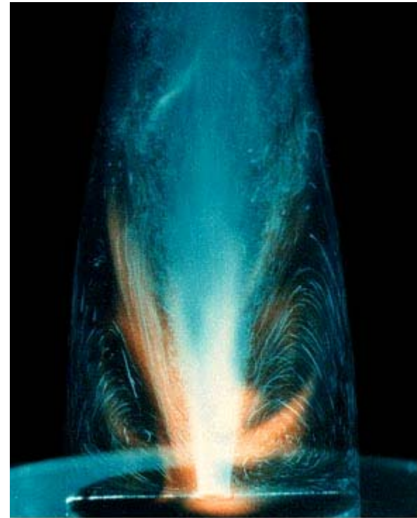
Jet flame with recirculation
