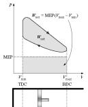
$$\begin{split} W_{net} &= \text{MEP} \times \text{Piston area} \times \text{Stroke} = \text{MEP} \times \text{DV} \\ MEP &= \frac{W_{net}}{V_{\text{max}} - V_{\text{min}}} = \frac{w_{net}}{v_{\text{max}} - v_{\text{min}}} \quad (kPa) \end{split}$$
