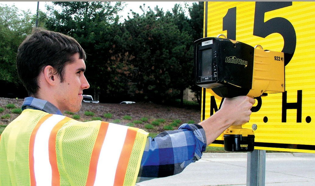
An LTAP undergraduate student measures the retroreflectivity of a street sign in West Lafayette. Retroreflective materials redirect the light from headlights back toward the vehicle.
