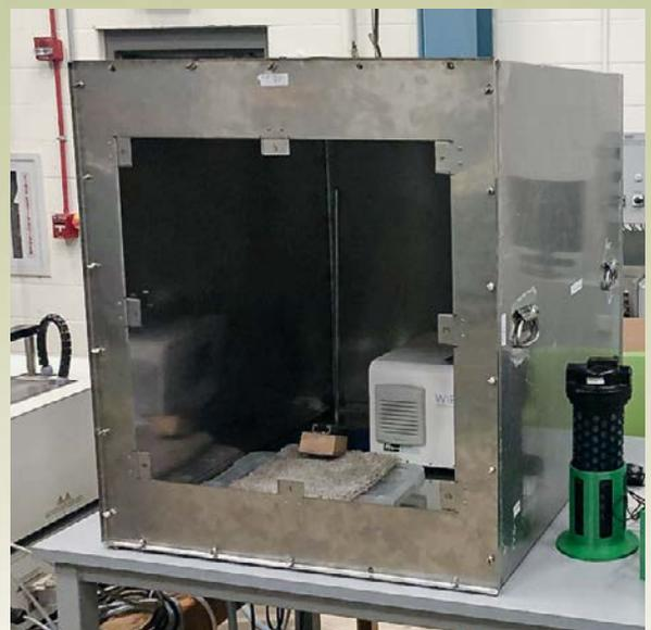
*Brian Magnuson, an undergraduate student researcher, helped design and build a full-scale environmental chamber to conduct dust transfer experiments.*
