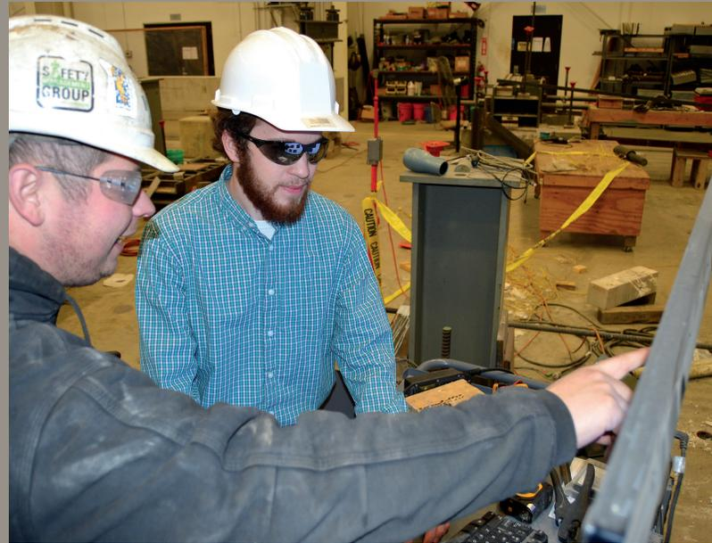
Bowen Laboratory project researcher Thomas Bradt and Purdue Civil Engineering undergraduate student Joshua Harmon examine load versus displacement data on web bending of a wide flange beam loaded in compression.
