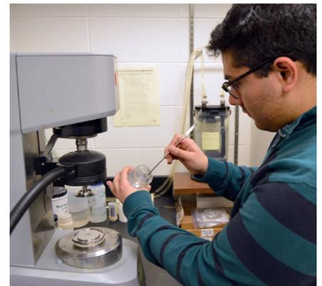
Lyles School undergraduate student Daniel Espinoza places a sample of the laponite gel onto the rheometer. A rheometer measures the way in which a sample flows in response to applied forces.
