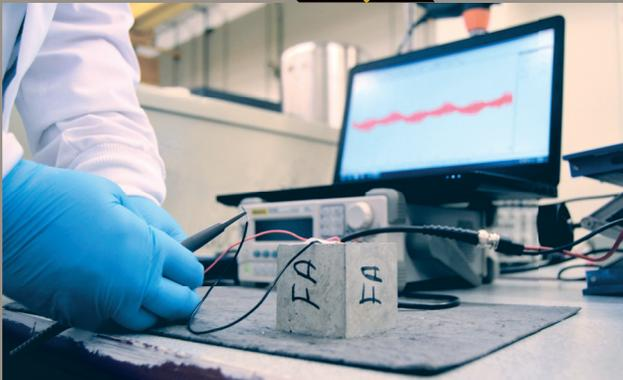
Associate Professor Na “Luna” Lu’s team uses piezoelectric sensors coupled with electromechanical impedance to determine early-age properties of concrete.
