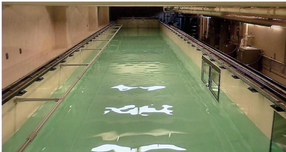
The towing tank, a 150-foot-long, 11-foot-wide and five-foot-deep water basin, will be used for coastal engineering and fluid dynamics research in the Burke Lab.
