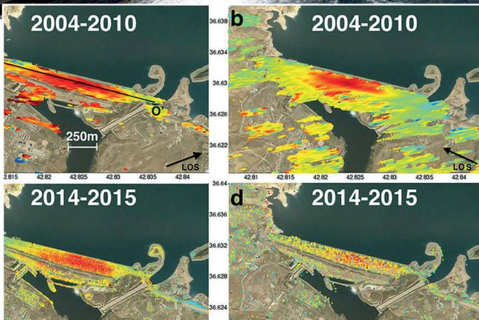
Perissin's team developed a multisensor cumulative deformation map for the dam based on satellite data. (Image source: Daniele Perissin, Nature.)
