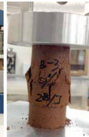
Specimen cylinder under loading. (Photo: Kuanchi Li)
