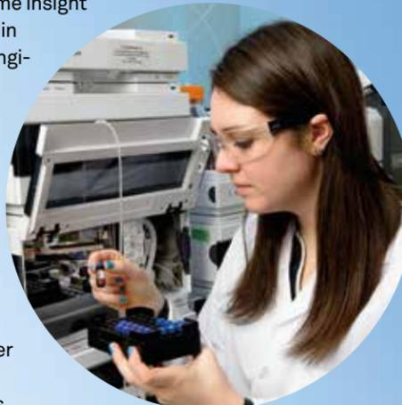
Holly Haflich puts nitrogen compound samples in the liquid chromatograph/mass spectrometry instrument, which separates and quantifies organic compounds.
