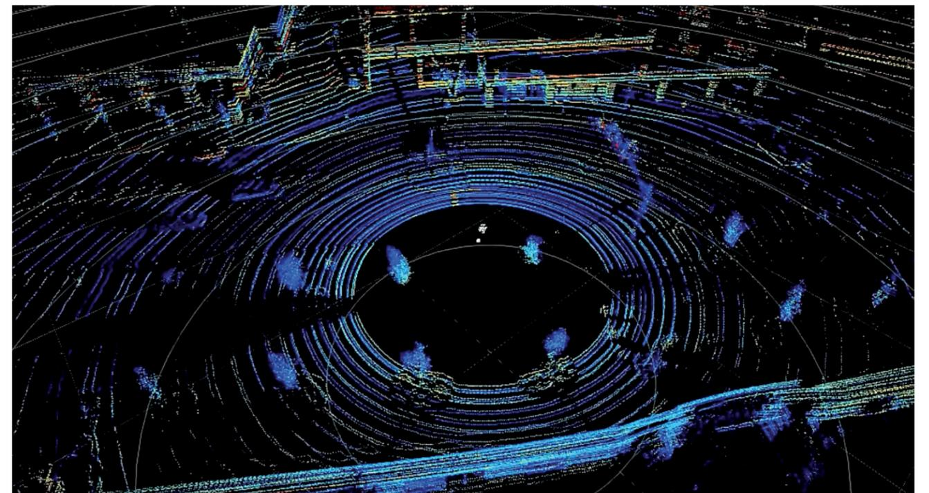
Purdue’s School of Mechanical Engineering is assisting in the study. Through a software program ME created, the raw data collected from the LiDAR technology is translated from countless dots on a black screen to a fully mapped traffic area, complete with data points that detail the speed of objects and pedestrians and their proximities to each other.
