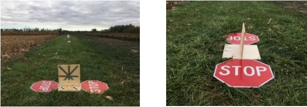
Figure 5. Calibration boards with reflective surface for aerial system
