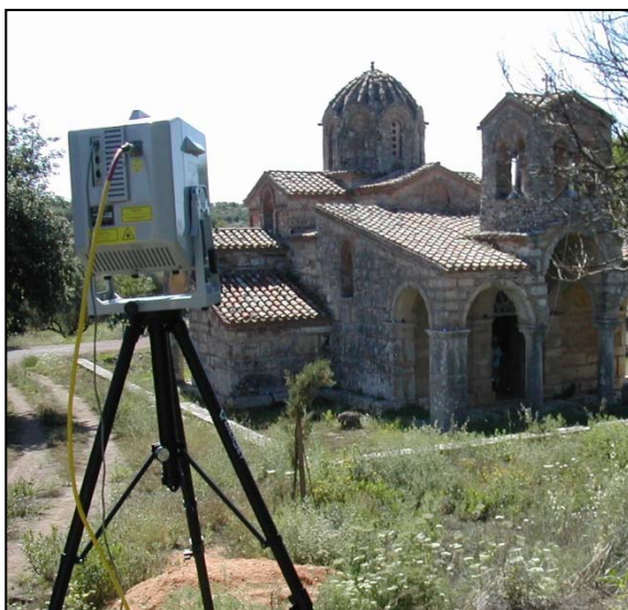
Static Terrestrial Laser Scanning
